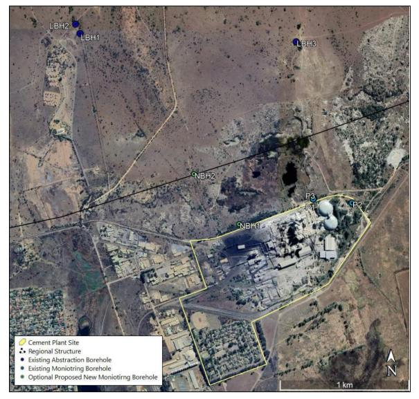
Figure 20: Cement Plant Groundwater Monitoring Network
