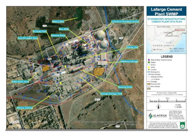
Figure 16: Lafarge Lichtenburg Cement Plant Proposed Stormwater Management Infrastructure
