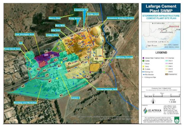
Figure 17: Lafarge Lichtenburg Cement Plant Proposed Stormwater Management Infrastructure Pollution Control Dam (PCD's)
